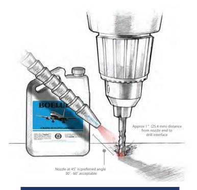
Using a coaxial supply of compressed air and lubricant to the nozzle, the nozzle directs BOELUBE<sup>®</sup> lubricant droplets in the compressed air directly to the cutting edge. The compressed air will help move chips from the tool cutting edge as the fine lubricant droplets form a thin film at the point of contact to reduce friction.
